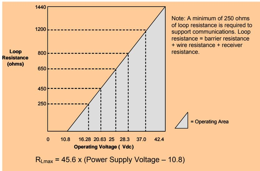
Figure 2 - Supply voltage and loop resistance chart & calculations
